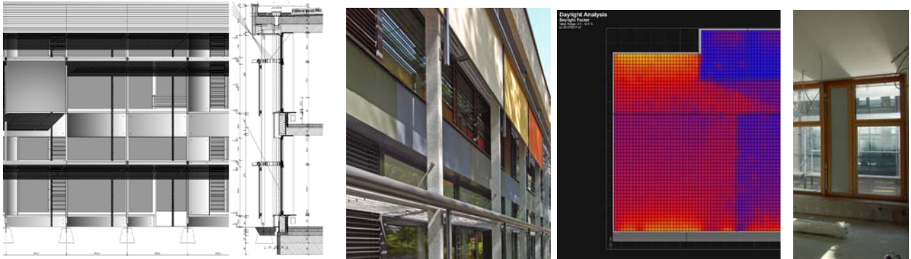
Fig. 6 South facade of the classrooms in detail, view from outside, calculated daylight factors (home area)
